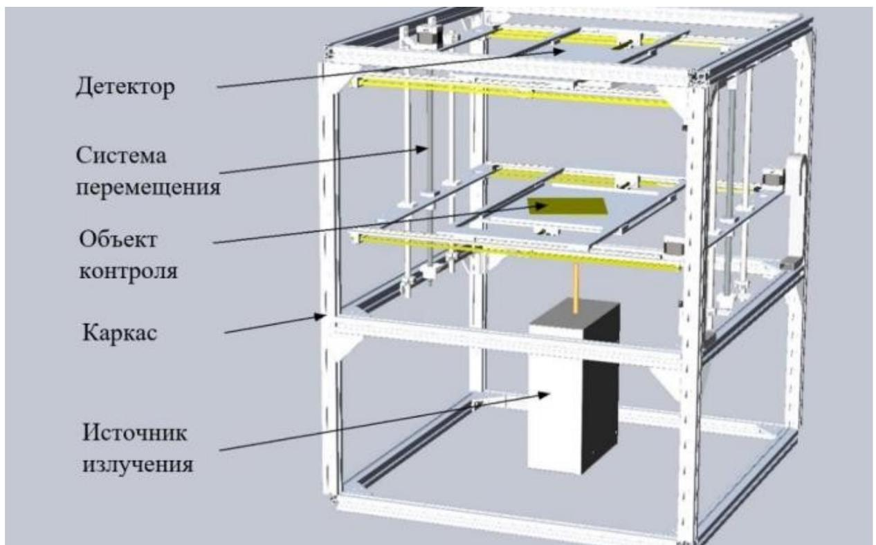
It looks familiar, doesn't it? Essentially it is a 3D printer with 5 axes in [CoreXY geometry](#).
