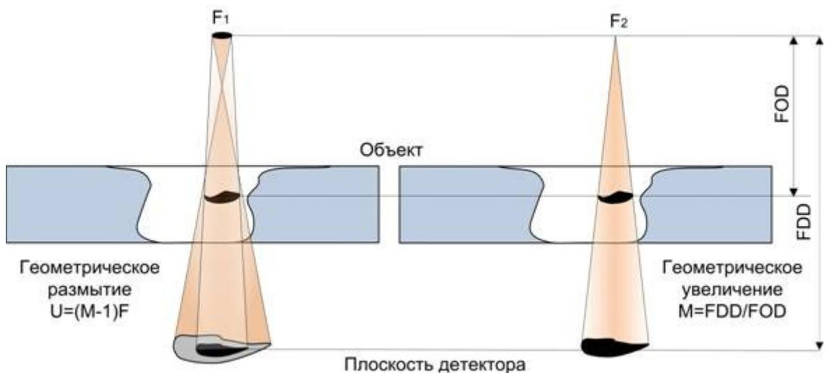
Object Geometric blurring  $U=(M-1)F$  Detector plane Geometric magnification  $M=FDD/FOD$
