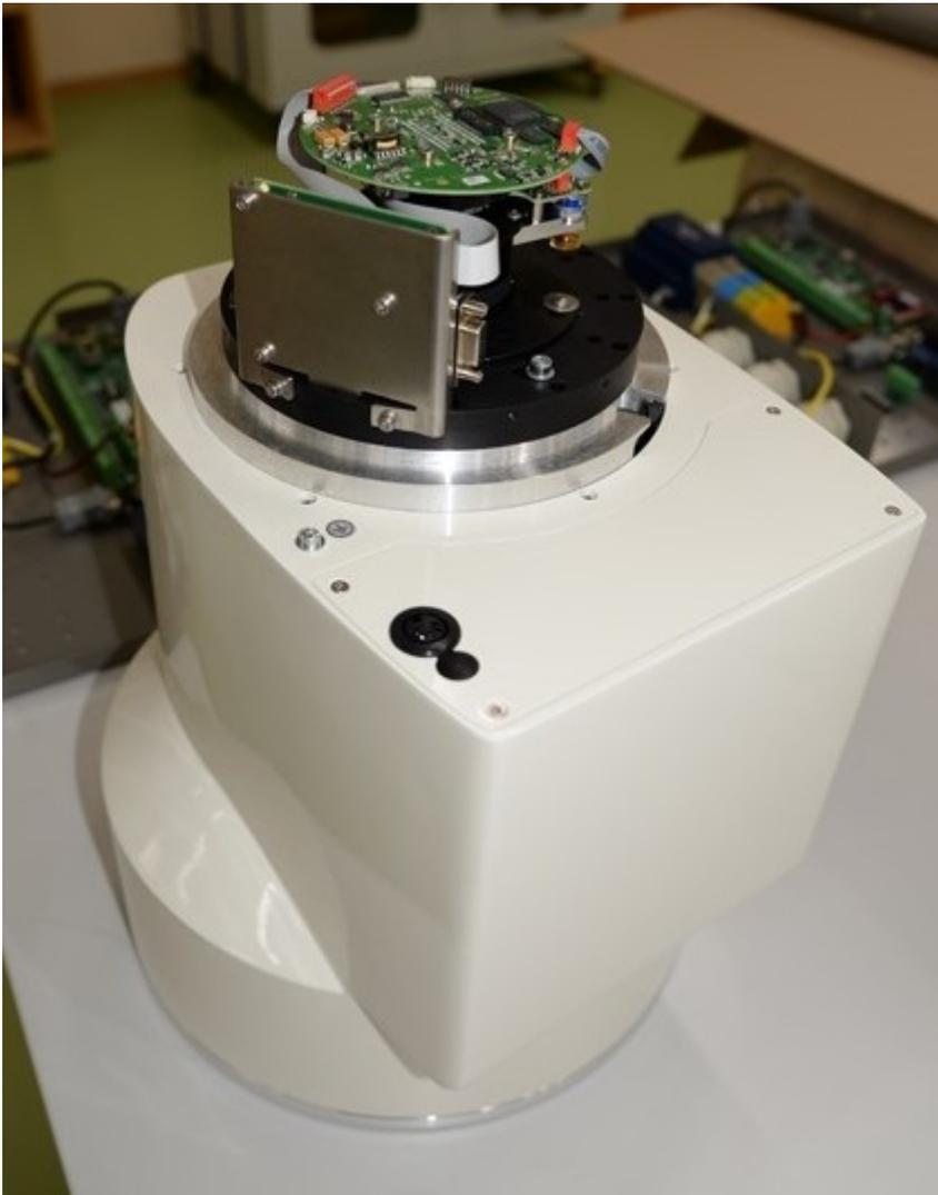
The next stage – detectors based on CCD matrices. Scintillator, optics and the sensor itself – they are already state-of-the-art. Advantage – high resolution, up to 2kx2k. Disadvantage – size of the CCD sensor is about 2x2 cm, let's remember photo cameras. They are used in microtomography as a low cost equivalent of flat panel detectors.
