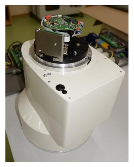
The next stage – detectors based on CCD matrices. Scintillator, optics and the sensor itself – they are already state-of-the-art. Advantage – high resolution, up to 2kx2k. Disadvantage – size of the CCD sensor is about 2x2 cm, let's remember photo cameras. They are used in microtomography as a low cost equivalent of flat panel detectors.
